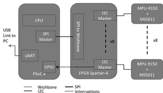
Figure 1: Centralized embedded motion system synopsis.
