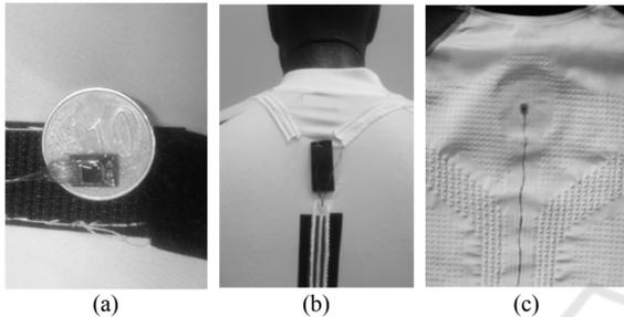
Figure 3: (a) New MPU9250 tags with thin wires, (b)(c) Sensors tags integrated into a t-shirt.
