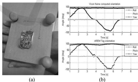
Figure 5: (a) AREM Gateway on a Vicon frame, (b) Roll orientation comparison with Vicon.
