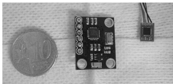
Figure 2: AREM v0 sensor tag (middle), AREM v1 sensor tag (right).
